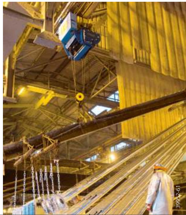
Semi-automatic monorail circuit with rope hoists in tandem operation
